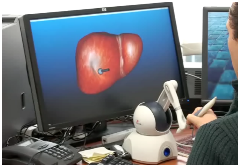
Fig. 8 – Liver palpation simulation at 850Hz haptic frame rate
